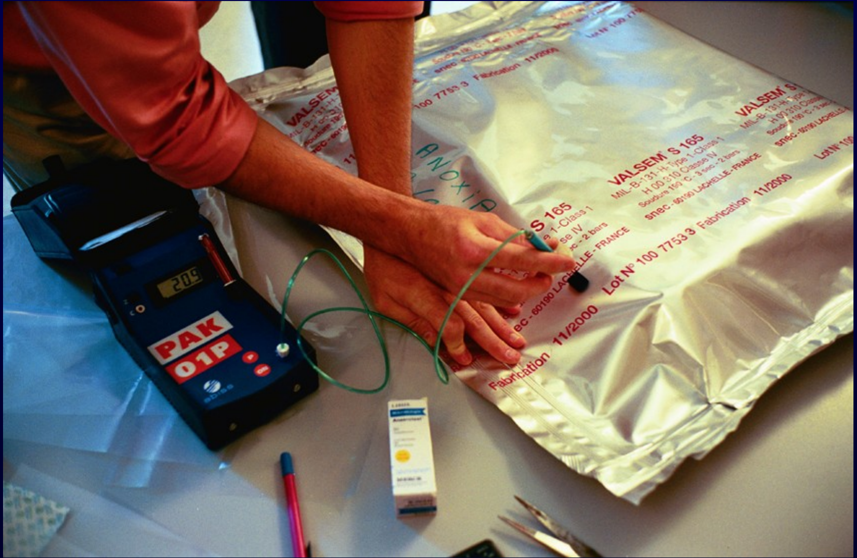
Placement of the oxymetre for the control of the oxygen loss in the bag.
